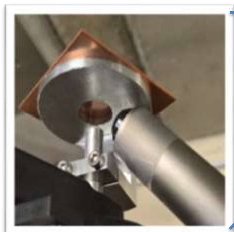
Details of the sample holder and collimator
