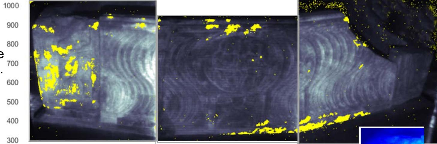
Additionally the presence of natural waxes was revealed in images collected at 415 nm
