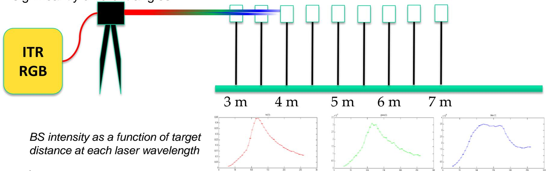
*BS intensity as a function of target distance at each laser wavelength*
