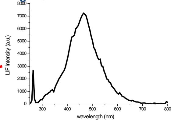
LIF spectra collected in the areas pointed by red arrow (LIF scanning prototype was used)
