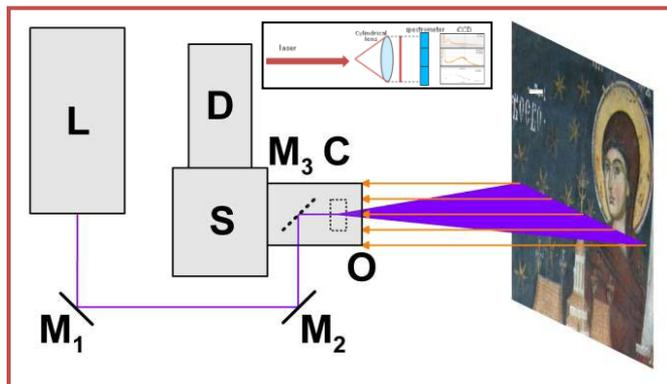
The laser beam is shaped as a light blade, thus there is no need to vary in-plane  $\theta$  angle, the scan system controls only the bending  $\varphi$ . The entire line profile is imaged on the monochromator slit, which spreads the entire spectrum collected at each point on the squared ICCD at  $90^\circ$ . **Time Resolved** data are obtained collecting **LIF spectra** at different delays, by gating the camera.
